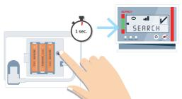
2 Press pair button for 1 second on base station. "SEARCH" appears on the display of base station.
