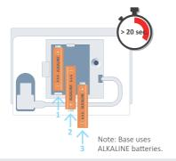
5 Replace the 3 base batteries within **20 seconds** – exchange one by one.
