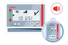
4 Once the sensor has been successfully paired, the sensor ID will appear on the display of base station for a few seconds, green LEDs will blink again, you'll hear a confirmation tone.
